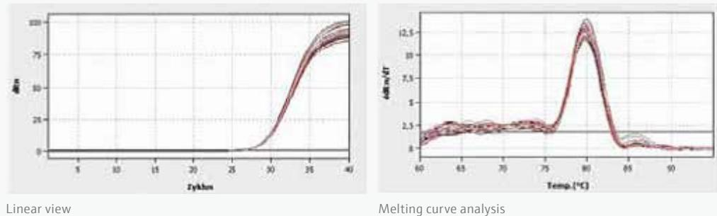
Also regarding to the used PCR reaction volume the qTOWER<sup>3</sup> shows an enormous capacity. In a range of 5  $\mu$ l to 20  $\mu$ l a standard deviation of only 0.07 for Ct values and 0.08 °C for melting temperature can be achieved.
