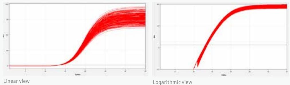
The single excitation and detection of each well avoids the often observed edge effects and allows excellent, homogeneous amplification plots over the entire 384 well block.
