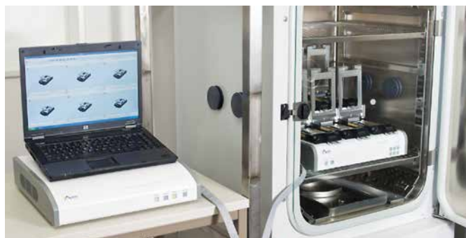
Figure 2: Cellular analysis under optimal environmental conditions ensures physiologically relevant results. RTCA Plate Stations* can be placed inside standard cell culture incubators (RTCA MP Plate Station is shown), creating a temperature-, CO 2 -, and humidity-controlled environment throughout an experiment.
